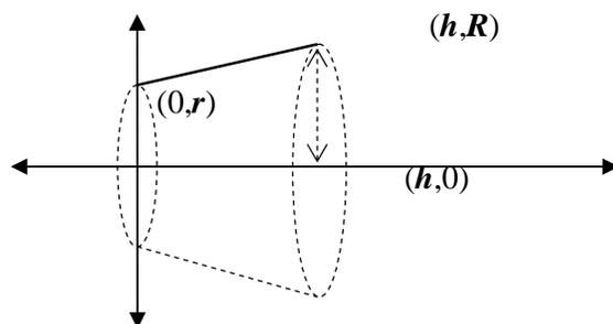
Fig. 2: Frustum with top and bottom bases at  $(0,0)$  and  $(h,0)$  respectively; and small and large radii of  $r$  and  $R$  respectively.
