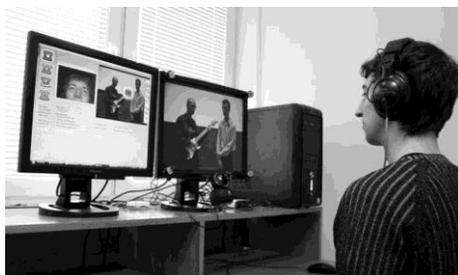
Fig. 3. Employing gaze tracking system during the experiment of audio-visual correlation (with stereo sound).
