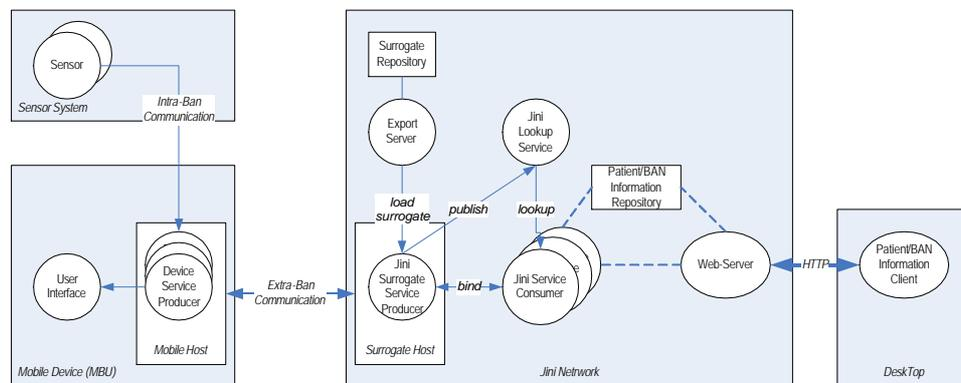
Figure 2: Overview of the Remote Patient Monitoring System based on Mobile Services Platform.
