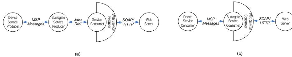
Figure 3: Service Integration: (a) integrating a device service producer; (b) integrating a device service consumer.
