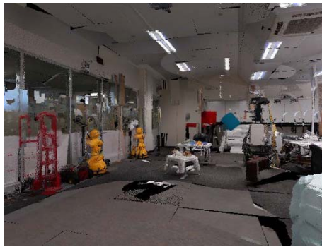
Figure 3. Riegl Laser Scan of Lab.
