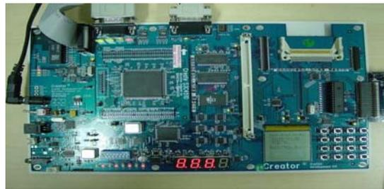
Fig. 6. Development Board of the Embedded Broker
