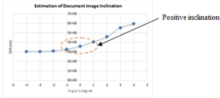
Fig. 4. An illustration for detection of text area inclination.
