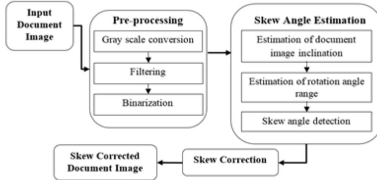
Fig. 2. Workflow diagram of skew detection and correction system.
