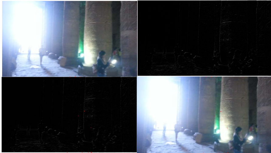
Fig. 5. Image capturing process in real-time improvements. From left to right and top to bottom: original frame, filtered, filtered with heuristic points, original with heuristic points.
