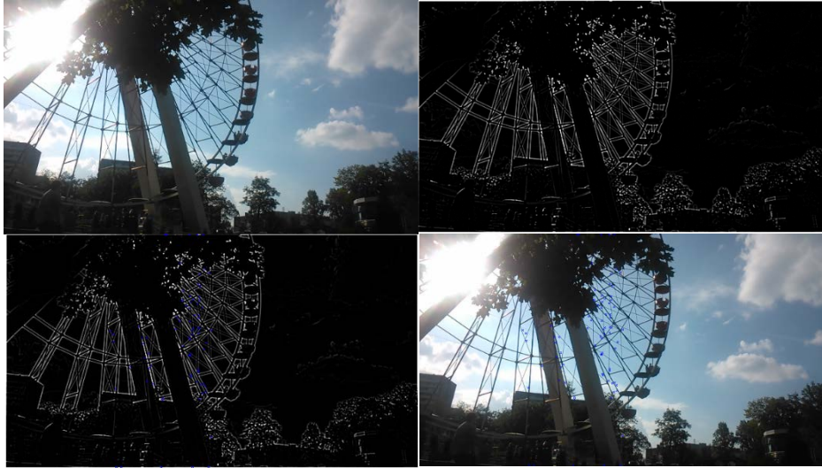
Fig. 3. Image capturing process of wheel in real-time improvements. From left to right and top to bottom: original frame, filtered, filtered with heuristic points, original with heuristic points.
