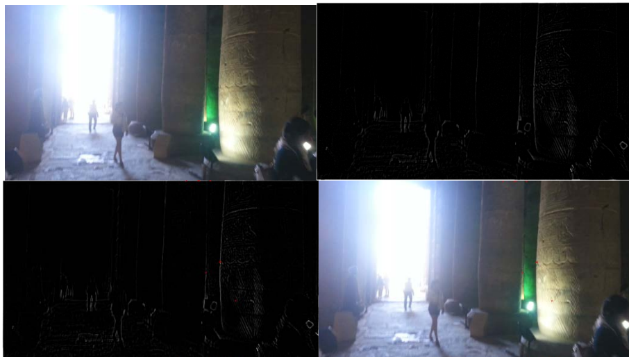
Fig. 6. Image capturing process in real-time improvements. From left to right and top to bottom: original frame, filtered, filtered with heuristic points, original with heuristic points.
