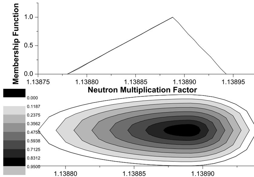
Fig. 4. MF of neutron multiplication factor and associated uncertainty
